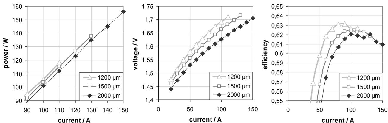
**Figs. 12** (left), **13** (middle) and **14** (right): Examples of electro-optical characterization of diode lasers with laser diode bar design H1 on active coolers for various resonator lengths: A section of the LI-curves (left), VI-curves (middle) and efficiency plots (right).
