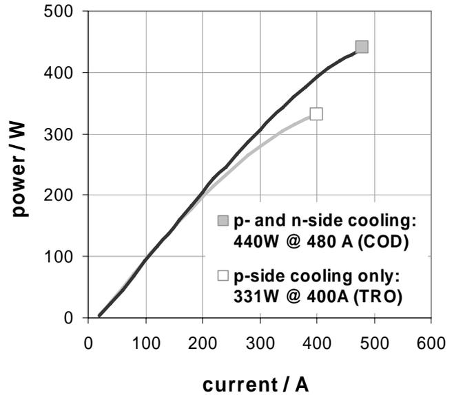
**Fig. 25:** Cw operation of diode lasers with *OSRAM* 940nm laser diode bars of 2mm resonator length (50% filling factor), mounted with indium solder on actively cooled heat sinks at output power limits at currents between 400 and 500A.
