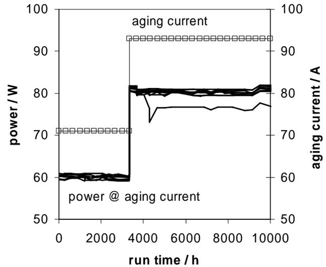
**Fig. 23:** Aging test of 9 diode lasers with *JDL* 940nm laser diode bars, 50% filling factor, 1.5mm resonator length, mounted with gold-tin solder, passively cooled, in hard-pulse operation mode of 0-71A / 0-93A 1s pulses at 0,5 Hz. Concerning the failure: see explanation in text above.
