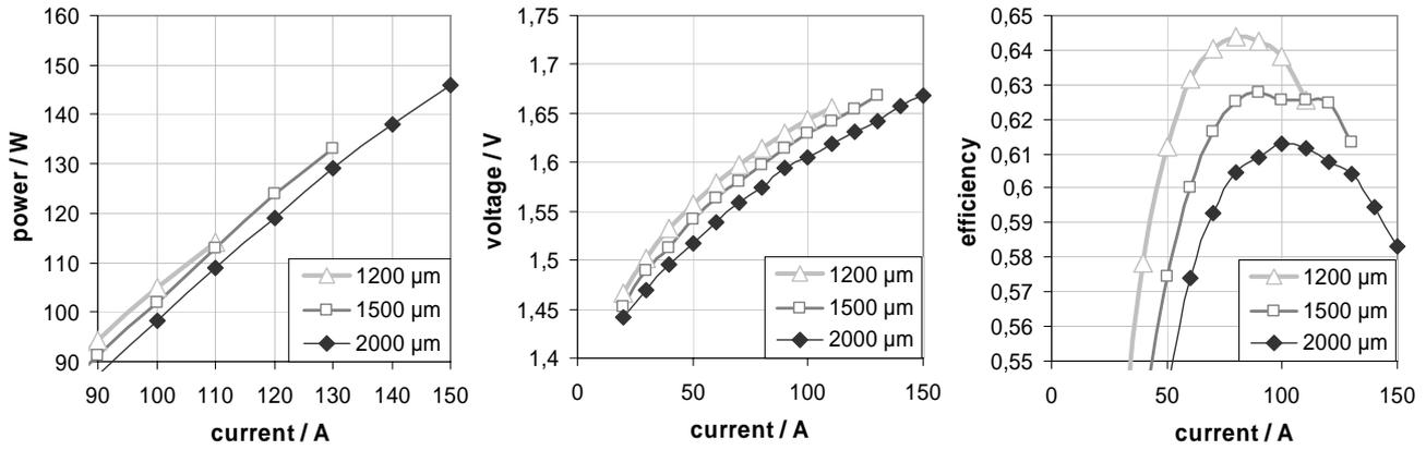
**Figs. 17** (left), **18** (middle) and **19** (right): Examples of electro-optical characterization of diode lasers with laser diode bar design H1 on passive coolers for various resonator lengths: A section of the LI-curves (left), VI-curves (middle) and efficiency plots (right).
