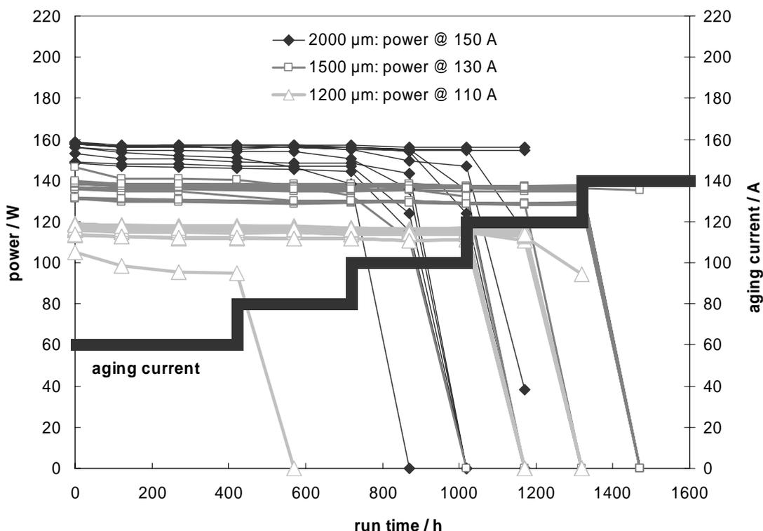
**Fig. 15:** Current-step failure discrimination test on 3 times 12 actively cooled diode lasers with indium-mounted laser diode bars. The optical output power has been measured every 150 h hours outside the aging test station at the currents mentioned for each resonator length.
