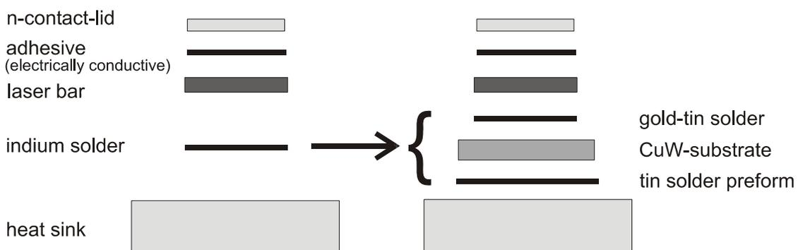
**Fig. 7:** The crossover of the standard diode laser packaging technology<sup>4,5</sup> at *JENOPTIK Laserdiode GmbH* from indium solder to eutectic gold-tin (80/20) solder. Expansion matching to the GaAs laser bar is achieved by the CuW-substrate, high thermal conductance through a copper heat sink, onto which the substrate is mounted by a tin solder preform.
