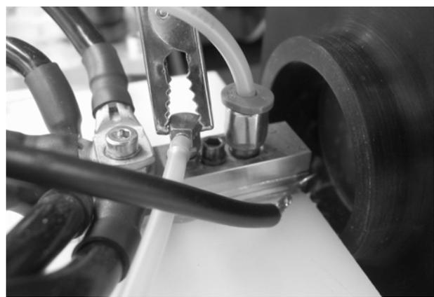
**Fig. 27:** Operation and measurement setup for double micro channel cooled diode lasers in front of power meter.
