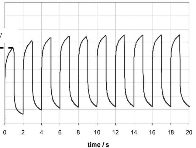
**Fig. 11:** FEM simulation result for the transient thermal behavior of 1200µm long diode laser bars in the passively cooled assemblies when operated at 1s pulses at 0,5 Hz.
