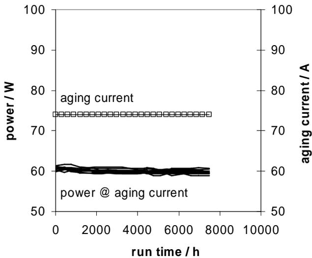
**Fig. 22:** Aging test of 12 diode lasers with *JDL* 940nm laser diode bars, 50% filling factor, 1.5mm resonator length, mounted with gold-tin solder, passively cooled, in hard-pulse operation mode of 0-74A 1s pulses at 0,5 Hz.
