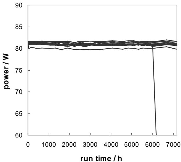
**Fig. 5:** Aging test of 12 diode lasers with JDL 940nm laser diode bars, 50% filling factor, 2.0 mm resonator length, mounted with indium solder, actively cooled, in soft-pulse operation mode of 15-91A 500ms pulses at 1 Hz. Concerning the failure: see explanation in text above.
