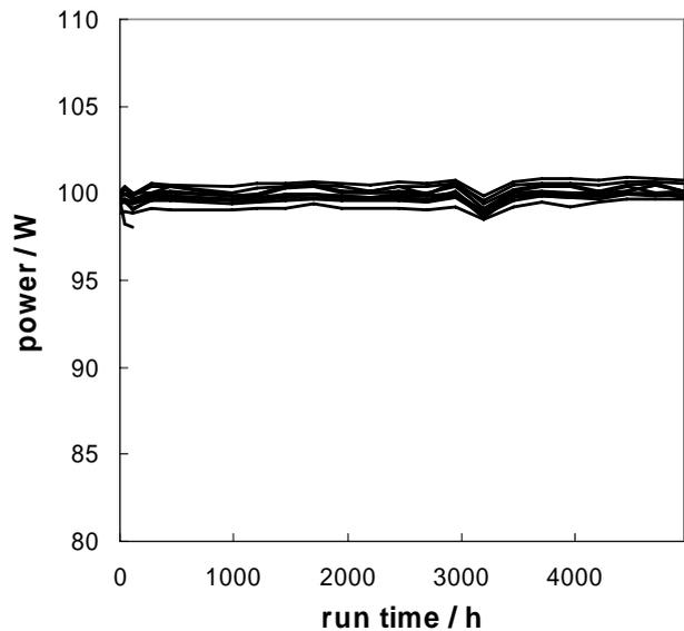
**Fig. 6:** Aging test of 12 diode lasers with JDL 940nm laser diode bars, 50% filling factor, 2.0mm resonator length, mounted with indium solder, actively cooled, in soft-pulse operation mode of 18-105A 500ms pulses at 1 Hz. Concerning the failure: see explanation in text above.
