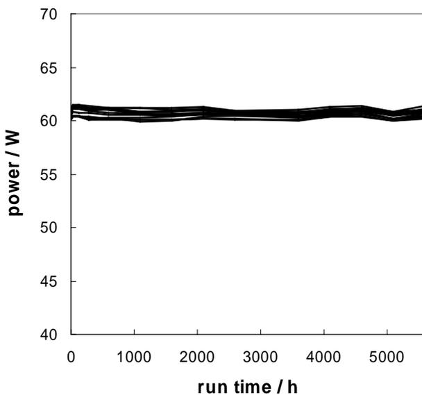
**Fig. 3:** Aging test of 12 diode lasers with JDL 940nm laser diode bars, 50% filling factor, 1.5mm resonator length, mounted with indium solder, actively cooled, in hard-pulse operation mode of 0-68A 500ms pulses at 1 Hz.
