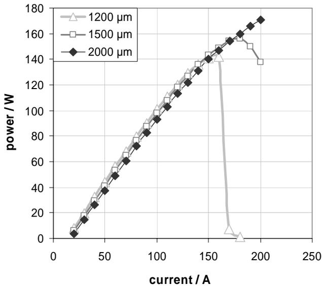
**Fig. 24:** Cw operation of diode lasers with *OSRAM* 940nm laser diode bars of various resonator lengths (50% filling factor) mounted with gold-tin solder on passive heatsinks, at optical output power limits around currents of 200A.
