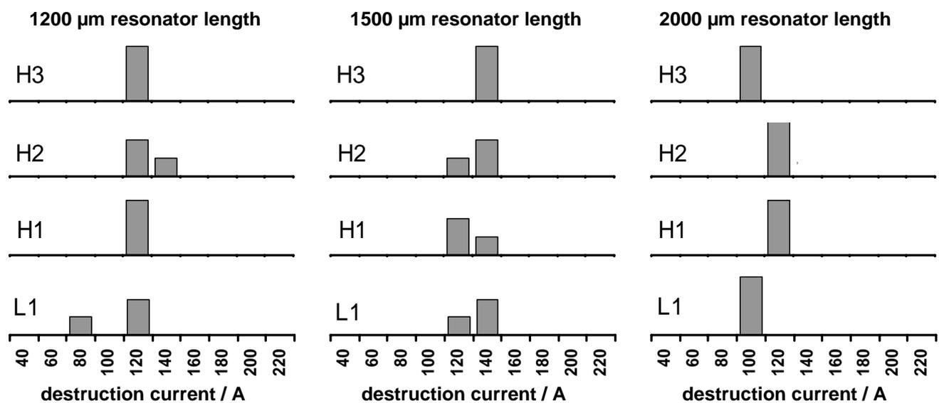
**Fig. 16:** Reliability histograms of the number lasers failed at the responsible destruction current for each laser design. The smallest block corresponds to one laser, the biggest to three lasers.
