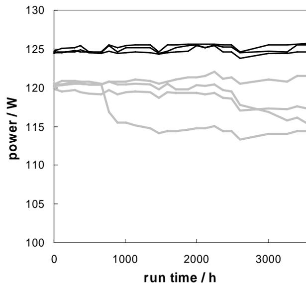
**Fig. 4:** Aging test of 7 diode lasers with JDL 940nm laser diode bars, 50% filling factor, 2.0mm resonator length, mounted with indium solder, actively cooled, in continuous-wave operation mode of 127A.
