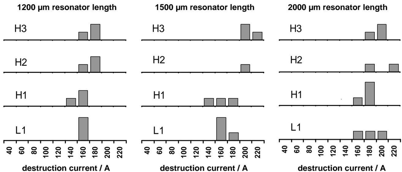
**Fig. 21:** Reliability histogramms of the number lasers failed at the responsible destruction current for each laser design. The smallest block corresponds to one laser, the biggest to three lasers.
