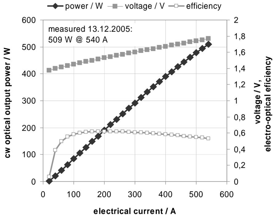
**Fig. 28:** Properties of a diode laser with a 3mm long *JDL* 940nm laser diode bar double-side micro channel cooled packaged with indium.
