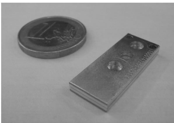
**Fig. 26:** *JOLDS* 500W diode laser with 3mm laser bar from *JDL* sandwiched between two copper micro channel coolers.
