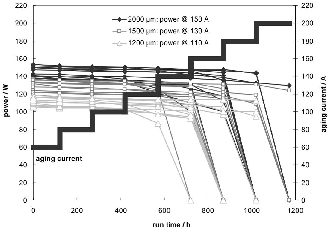
**Fig. 20:** Current-step failure discrimination test on 35 passively cooled diode lasers with gold-tin-mounted laser diode bars. The optical output power has been measured every 150 h hours outside the aging test station at the currents mentioned for each resonator length.
