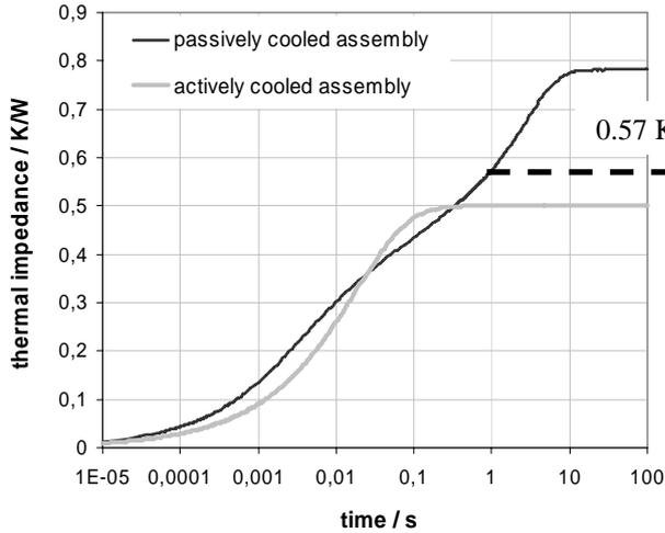
**Fig. 10:** FEM simulation results for the transient thermal behavior of 1200µm long diode laser bars in the actively and passively cooled assemblies in the first 100s of cw mode.
