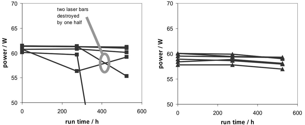
**Figs. 8 (left) and 9 (right):** Results of a first comparative study of 12 passively cooled diode lasers, where 6 laser diode bars were soldered with indium (left) and 6 with eutectic gold-tin (right). The diode lasers with 940nm JDL laser diode bars of 50% filling factor and 1500 $\mu$ m resonator length were operated in hard-pulse mode. Three indium soldered lasers failed within 500h of operation, whereas all gold-tin soldered lasers remained unaffected.
